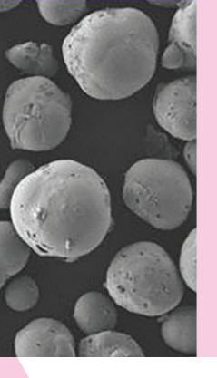
Perlite products are made from a volcanic rock which contains 2-6% water in its inner structure. When heated to around 900°C, the water trapped within the structure is vaporized, causing the material to expand and form a spherical structure.
